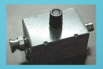
Uses a small frequency generator to mix with the "fox" frequency, and you listen to the mixing product
