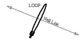
The Loop Antenna has the advantage of being less affected by reflection signals due to its Faraday shield.
